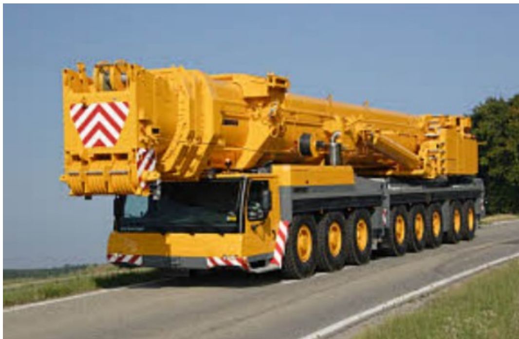
Plate 4.6: Crane for wind turbine erection 2
